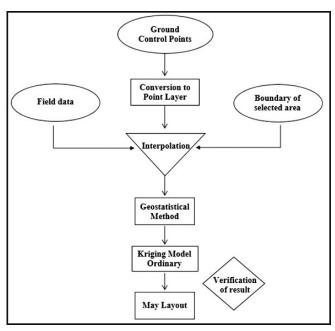
**Fig. 3.** Flow chart of Kriging Interpolation method. This figure shows the overall procedure adopted to interpolate a raster surface from collected ground points. Interpolation process allow to estimate and predict unknown value from a known geographic point data within a specified distance. This method was adopted to estimate the spatial distribution of feral horses in the study area.
